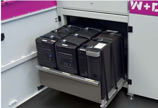
RIP, data transfer and print head control
